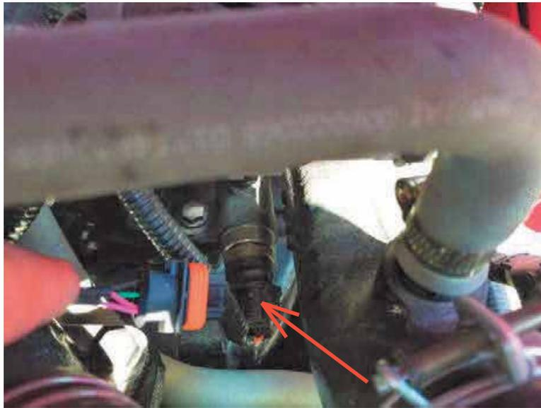
**3)** Looking directly over the top of the engine locate and unplug the 4 individual injector connectors. You will want to start at the back of the engine (firewall side) with injector connector "A" and work your way toward the engine fan ending with injector connector "D".
